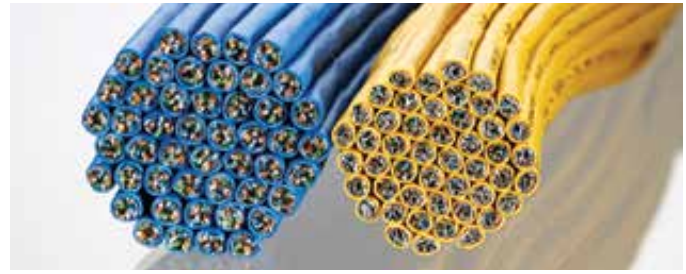
Figure 3: Comparison of 26 AWG (left) and 28 AWG (right) DataMax® patch cord cable. DataMax® Mini 6a F/UTP 28 AWG patch cord cable is 23% smaller in size, 38% smaller in cross-sectional area and 33% lighter than standard 26 AWG cable.
