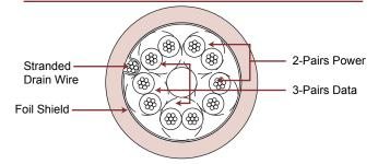
Data pairs: foam polypropylene Power pairs: solid polypropylene Data pairs' impedance 100 +/- 10 Ohms to 300 MHz Design developed using length and data rate
