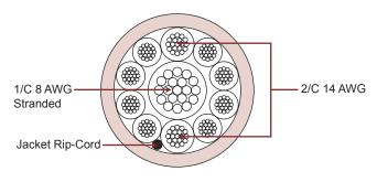
8 AWG for power/grounding Core design for round, flexible cable without fillers 2/C 14 AWG and 8/C 16 AWG
