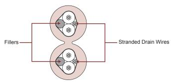
2-pairs 26 AWG foam insulated Foil shields bonded to jacket 110 Ohm impedance Pressured PVC "zip-cord" jacket
