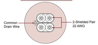
Common-axis cabling reduces size PVC or polyurethane pressured jacket Jacket provides sealed connection
