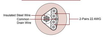
Pairs with common foil shields Rope-stranded steel strength member Pressure extruded polyurethane jacket
