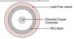
Cost-saving replacement for FEP designs Electrical/dimensional equivalent to RG-316 Fits RG-316 connectors 75 C maximum rating Other "RG" equivalents available
