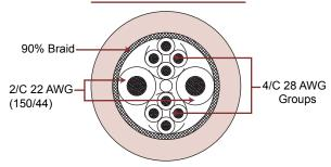
Flexible matte finished jacket Ultra-flexible stranded copper 40 AWG braid
