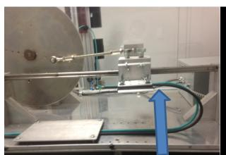
8. When top clamp is at full travel to the right, it is important to notice that there is no stress on the top cables where they meet the clamp.
