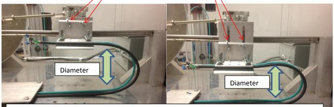
7. It is important to adjust the top clamp to the right diameter. The diameter of the setup can be calculated by taking the O.D. of the smaller cable and multiplying it by 20 for 10X flex testing. The diameter for 20X flex testing can be calculated by taking the O.D. of the smaller cable and multiplying it by 40. The top clamp can be adjusted to the required diameter for the 10X and 20X cables.
