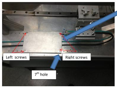
5. Bottom clamp should begin on the 7<sup>th</sup> hole from the right. Tight the 2 left screws simultaneously as well at the 2 right screws. STOP when a small resistance is given on the screws. A small space of about a third of an inch should be left between the two cables insuring that there is no contact. It is also important not to crush the cables with the plate by screwing it too tight.
