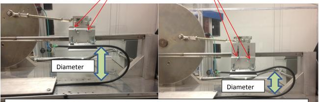
7. It is important to adjust the top clamp to the correct diameter. The diameter of the setup can be calculated by taking the O.D. of the cable and multiplying it by 20 for 10X flex testing. The diameter for 20X flex testing can be calculated by taking the O.D. of the cable and multiplying it by 40. The top clamp can be adjusted to the required diameter for the 10X and 20X cable.
