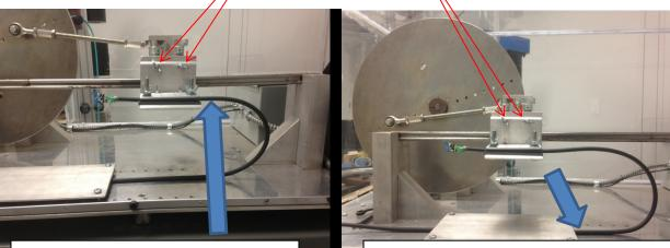
8. When top clamp is at full travel to the right, it is important to notice that there is no stress on the top cable where it meets the clamp.
