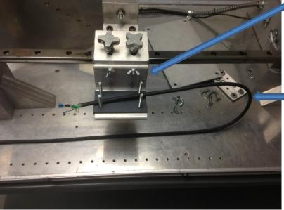
3. The inserted cable should 'flow' freely when inserted in the machine. When placed in the machine, the cable should relax without any tension. The natural twist of the cable lay should agree with its placement.
