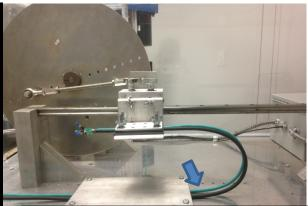
When top clamp is fully travel to the left, it is important to notice that there is no stress on the bottom part of the cables in where they meet the clamp.
