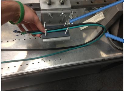
3. The inserted cables should 'flow' freely when inserted in the machine. The natural twist of each cable lay should agree with its placement.
