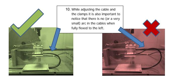
After the cable or cables are fully secure in the machine, electrical testing can begin. The two tests that are to be performed on each cable are "Return loss" (RL) and "Cross Talk" (NEXT). It is important to first electrically test the cable or cables before flex testing is done. When turning ON the machine the power cord can be plugged in.
