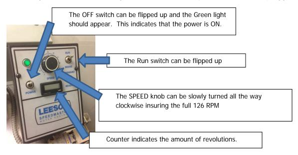
When the machine begins to turn and flex the cable, the access door is to be shut and locked for safety. Finally RL and NEXT testing can begin.
