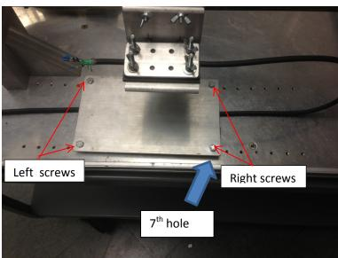
5. Bottom clamp should begin on the 7<sup>th</sup> hole from the right. Tighten the 2 left screws simultaneously as well at the 2 right screws. STOP when a small resistance is given on the screws insuring no crush on the cable.
