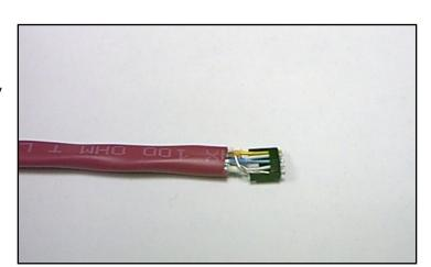
**Step 7** With the plug's release trigger positioned downward, and the orange conductor positioned leftmost, press the cable with load bar into the plug cavity causing the leads to now extend to the far end of the plug nose.
