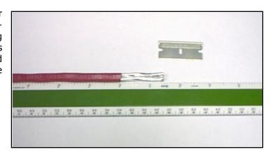
**Step 2** Remove all tapes flush with the jacket line. (**Tip**: A simple nick at the lip of each tape will permit easy tearing around the film. This is a very simple process.)
