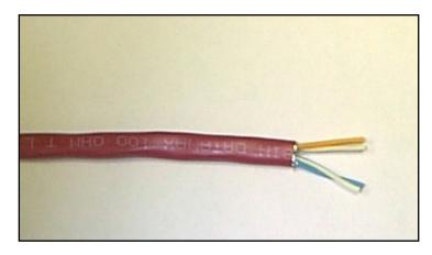
**Step 3** The insulation system of this construction is made up of a dual layered composite. Removing the outer layer (foam) will leave the inner insulation behind. Remove the outer insulation of all four leads leaving the inner insulation adhered to the copper wire.
