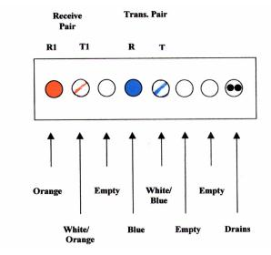
**Step 5** Slide the loaded "load bar" toward and flush with the jacket. Measuring from the jacket's edge, cut the extended leads and drains straight across and evenly leaving 5/8 inch.
