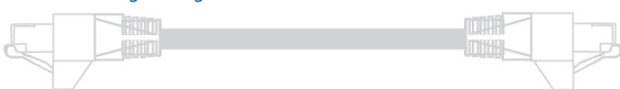
Examples based on 23 AWG Horizontal cable being used in each channel. TIA example utilizes 26 AWG patch cable.
